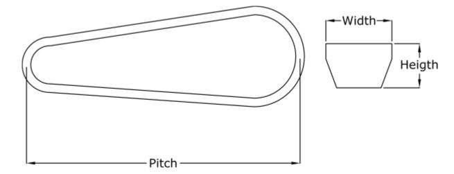
$\begin{array}{ll} \text{Datum Llength} = 5915 \\ \text{Height} &= 10 \\ \text{Length inside} &= 5855 \\ \text{Type} &= \text{BB230} \\ \text{Width} &= 17 \end{array}$
